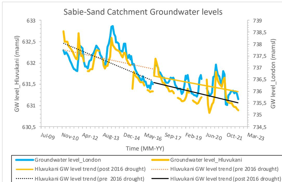
Fig. 1 A groundwater hydrograph from two boreholes in the Sabie-Sand showing sustained groundwater level decline post the 2015/2016 drought
