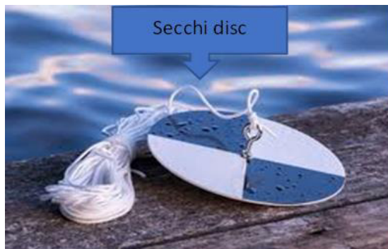
Figure 10: Secchi disc used to measure clarity.
