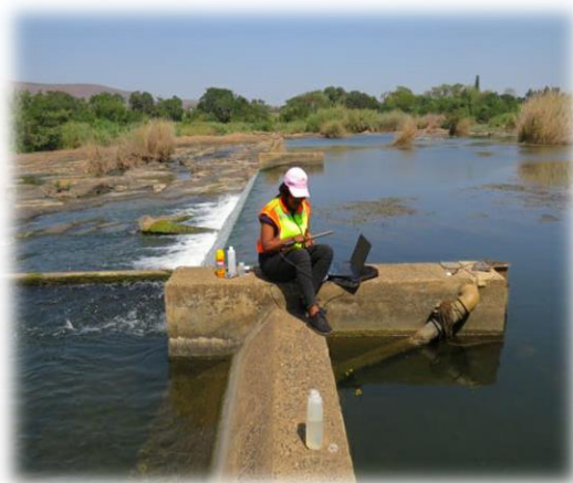
Figure 5: IUCMA official downloading data from probe through Win-Situ software.
