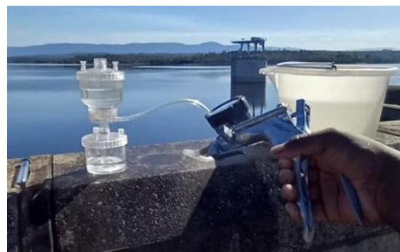
Figure 8: Filtration of Suspended solids or chlorophyll-a sample(s).
