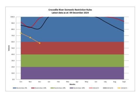
Figure 1: Operating rule curve for Kwena Dam: Restriction levels for domestic water use.
