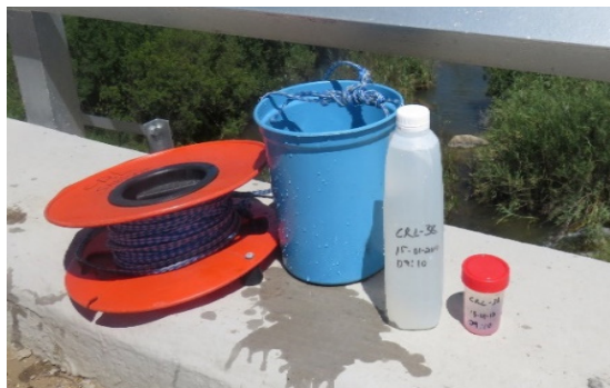
Figure 3: Chemical and Microbiological samples taken at Komati River downstream of Vygeboom Dam at R38 bridge using the bailer and the bucket
