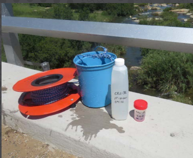
Figure 3: Chemical and Microbiological samples taken at Komati River downstream of Vygeboom Dam at R38 bridge using the bailer and the bucket
