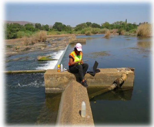
Figure 5: IUCMA official downloading data from probe through Win-Situ software.
