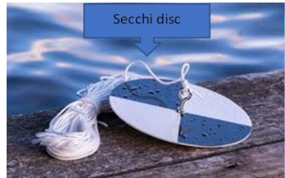
Figure 10: Secchi disc used to measure clarity.
