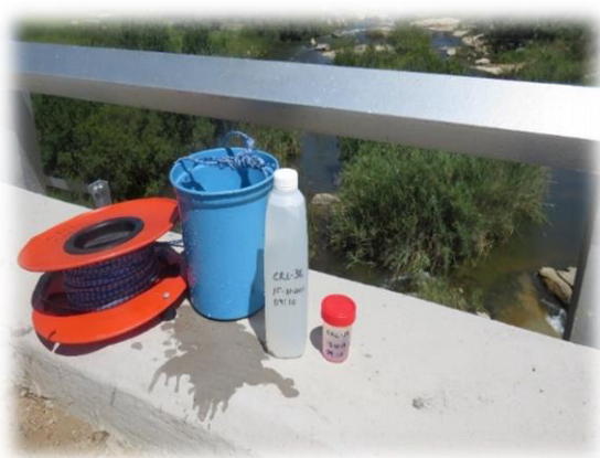
Figure 3: Water quality samples taken at Komati River using the bailer and the bucket.
