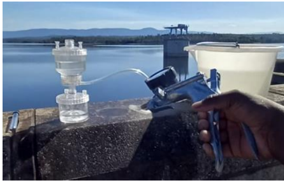
Figure 8: Filtration of Suspended solids or chlorophyll-a sample(s).
