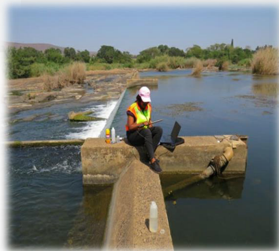
Figure 5: IUCMA official downloading data from probe trough Win-Situ software at Komati River.
