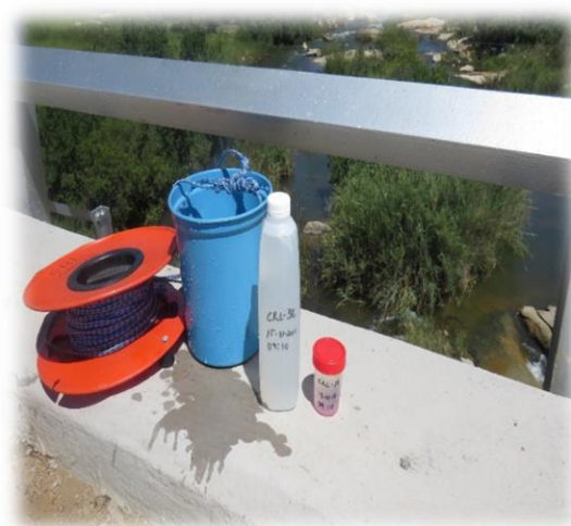
Figure 3: Chemical and Microbiological samples taken at Komati River downstream of Vygeboom Dam at R38 bridge using the bailer and the bucket
