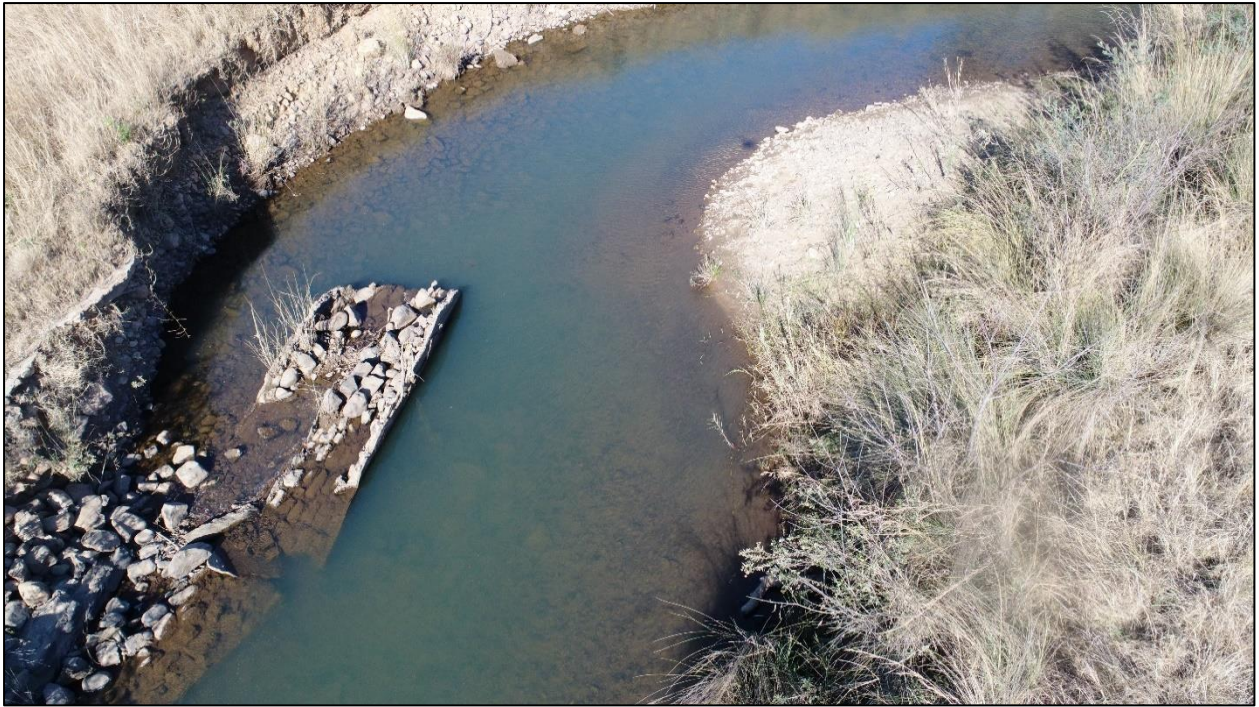
Figure13: Bank instability in the Crocodile River at EWR 2: X2CROC-GOEDE.
